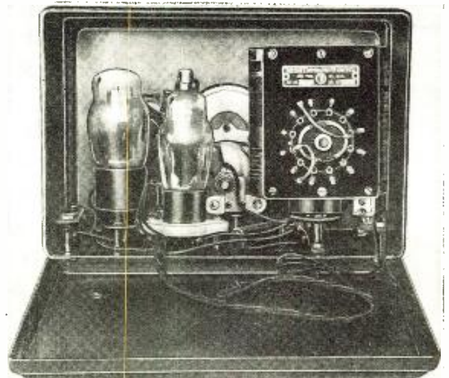
Photo above shows a rear view of the 2-volt receiver, which covers 16 to 550 meters with a handy hand-switch.
